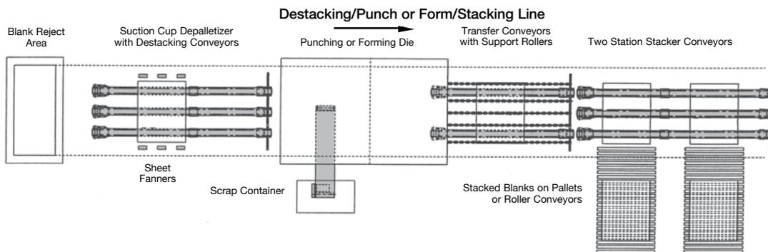
Bunting Stacking Conveyors eliminate one of the most common bottlenecks in metal-forming operations by providing an automated alternative to the manual stacking of sheet metal components as they come off the production line. Ruggedly built Bunting Conveyors can be used to move sheets or blanks directly from punch presses
